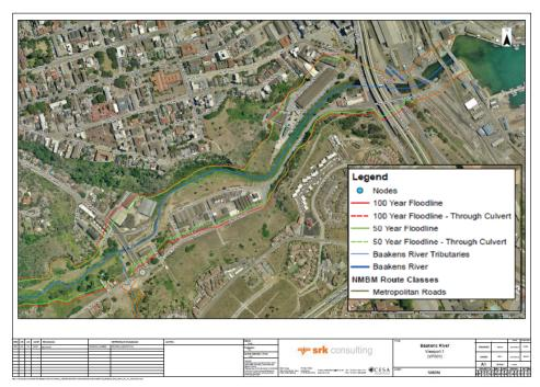
Figure 2.8 1:50 and 1:100 year floodlines for the Lower Baakens produced by SRK Engineers in 2014
