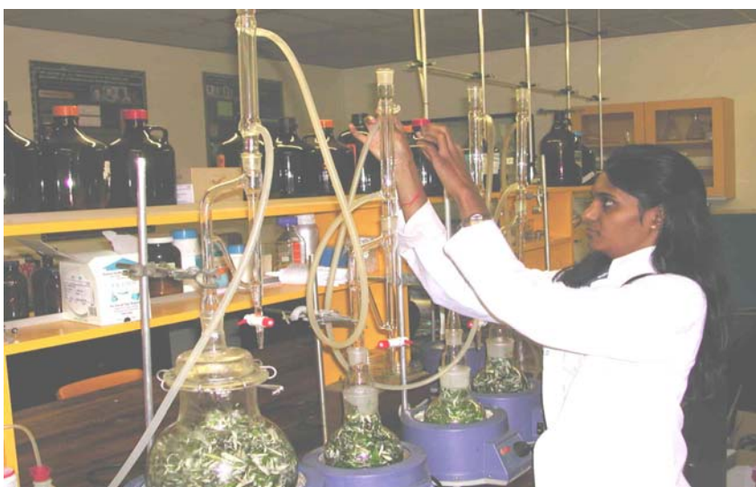
Figure 2.1: Hydrodistillation of plant material using the Clevenger-type apparatus.
