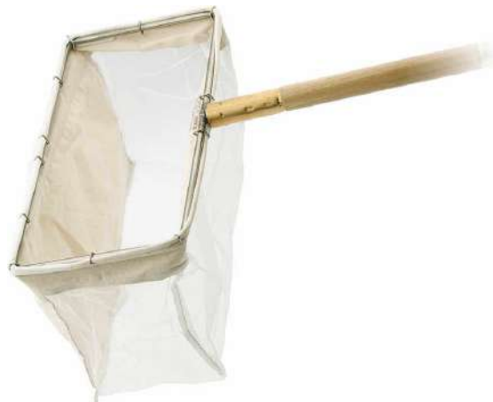
Figure 13. Kick net with 1 mm mesh used to dig through silt, sand, gravel substrates to depths of approximately 5 cm
