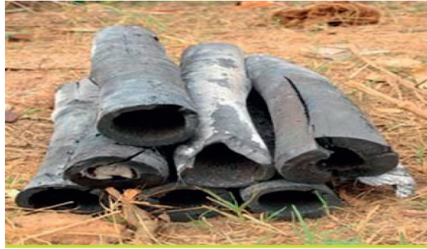
FIGURE 9: Bamboo charcoal making in Ethiopia (source: [22]).
