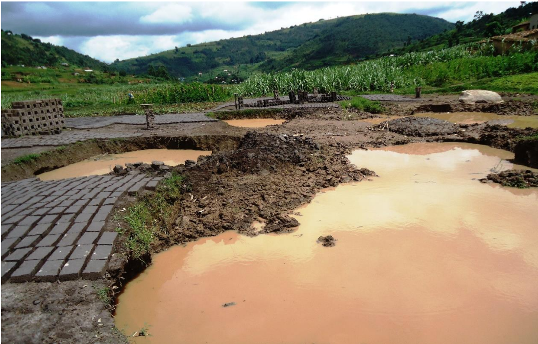
FIGURE 2-69: ORGANIC SOILS USED FOR BRICKS PRODUCTION IN RULINDO DISTRICT, NYARUBUBA WETLAND (PICTURE: MAY 2020)
