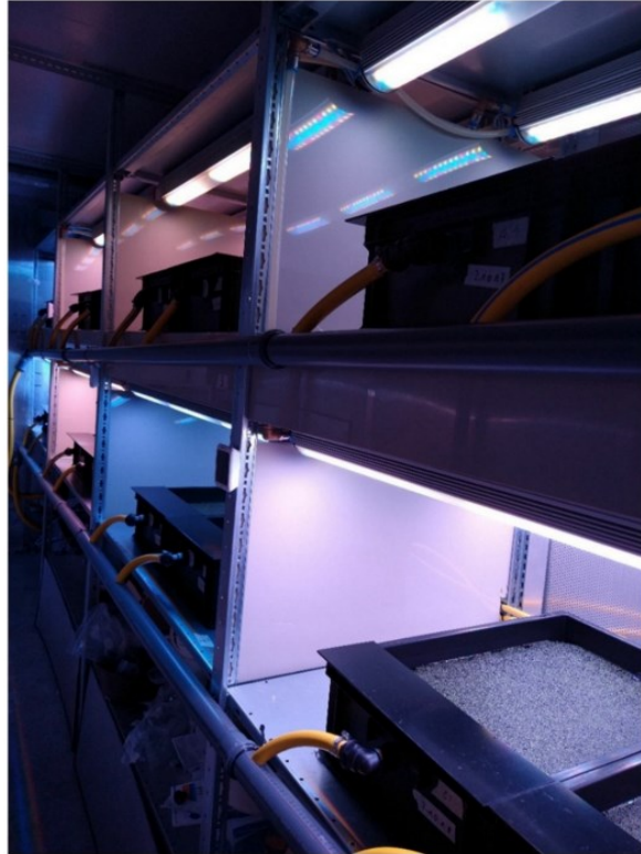
Figure 2. Experimental set-up in the container at the Osnabrück University of Applied Sciences, Germany. The light colors of the different spectral treatments are visible.
