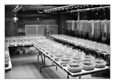
Figure 1. Set-up showing direct application of seedling emergence method in an environmental growth chamber at the US Army Engineer Research and Development Center (ERDC), Vicksburg, Mississippi.
