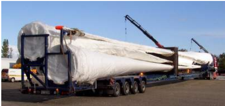
Figure 2: Example: 3 x 45m Blades on extendible trailers
