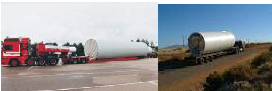
Figure 4: Transporting the Tower Sections
