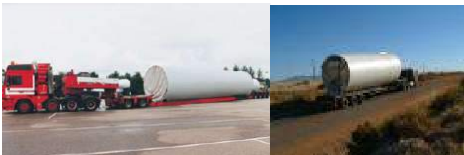
Figure 4: Transporting the Tower Sections
