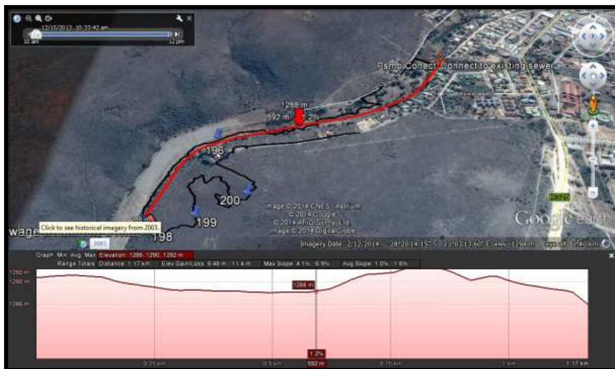
Figure 3: Google image showing the pipeline elevation from Pump station 1 towards the WWTW
