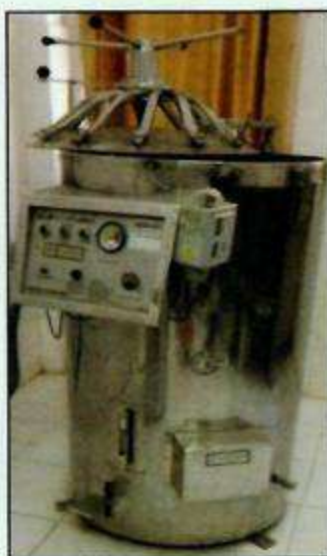
Vertical autoclave used for media preparation
