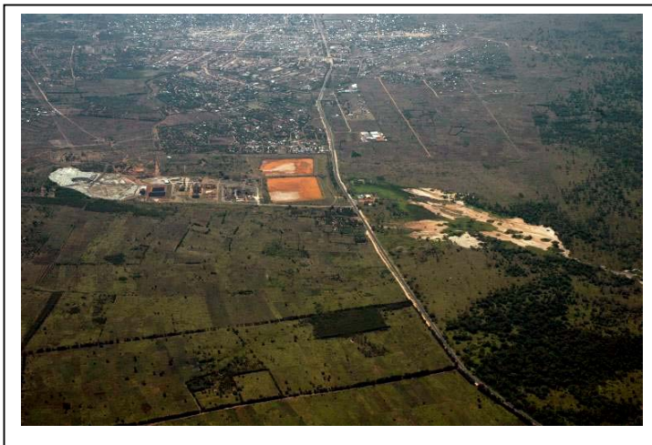
Figure 3.5. Cobalt slurry pond to left of Kasese Road with bare earth in QEPA to the right resulting from heavy metal pollution.
