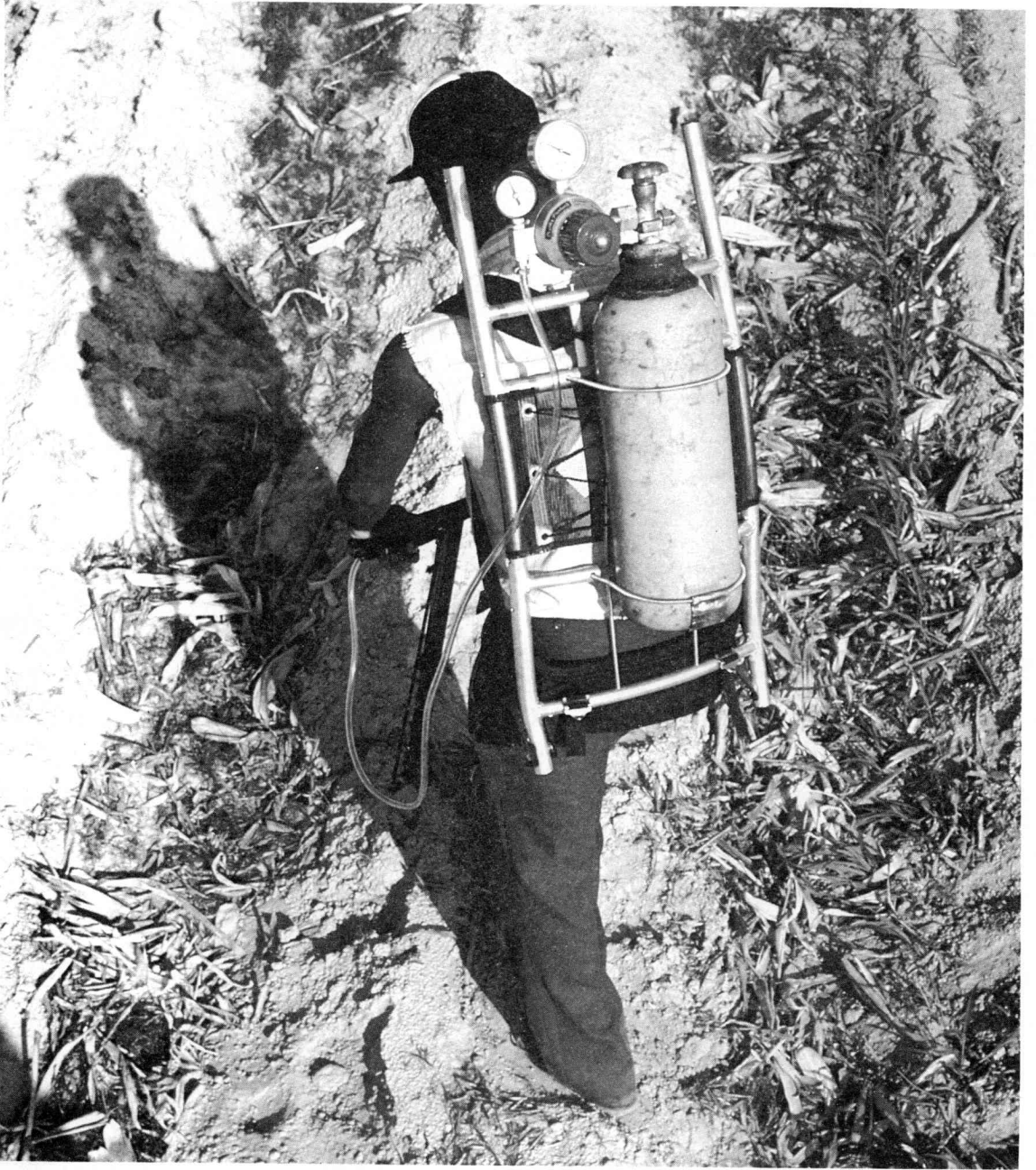
Slide 1 : Portable ethylene compound applicator in use in Striga -infested fields in the USA
