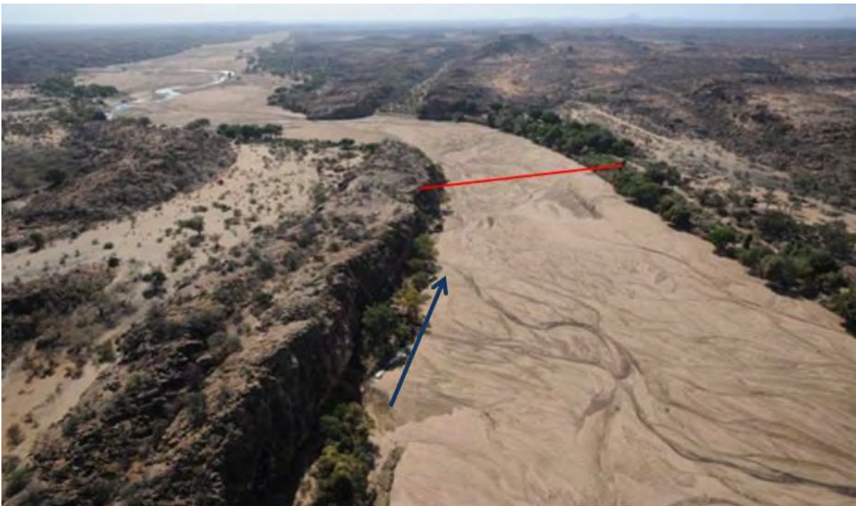
FIGURE 4.21: OBLIQUE AERIAL VIEW OF THE LIMPOPO RIVER AT THE POACHERS CORNER SITE. THE CROSS SECTION AND FLOW DIRECTION ARE INDICATED ON THE IMAGE
