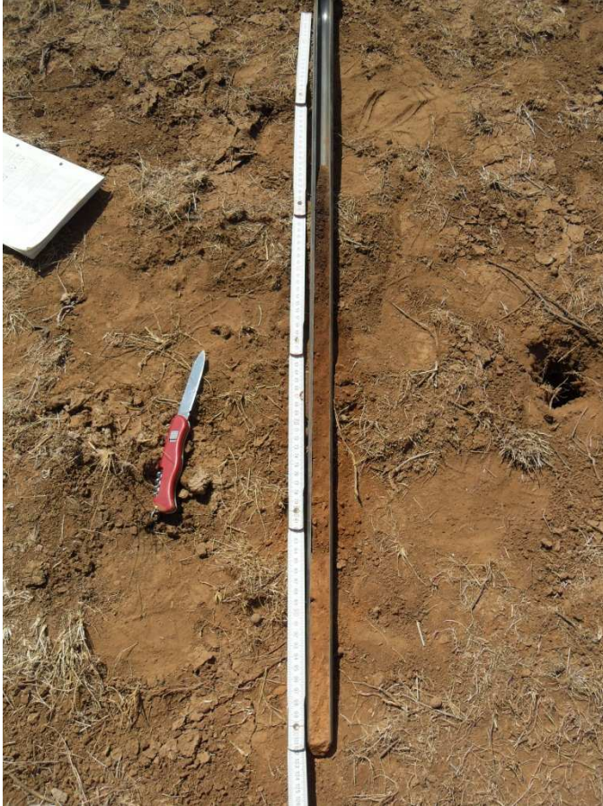
Pic 6: Puerckhauer auger for soil sampling
