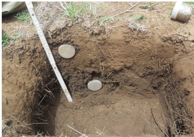
Pic 5: Setup of bulk density determination site
